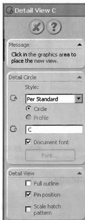
Slika 13-33 Pano Detail View PropertyManager
